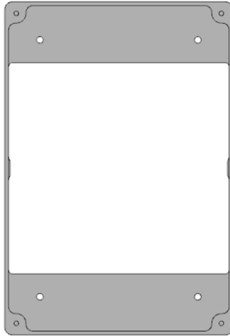
Figure 8: Interior of Heater Block Subassembly Housing
