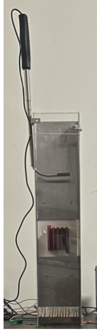
Figure 15. Built Vertical Enclosure with Heater Block Subassembly
